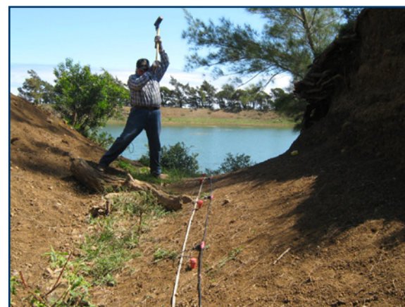
Preparing to swing a 12-pound sledge hammer to create a seismic wave
